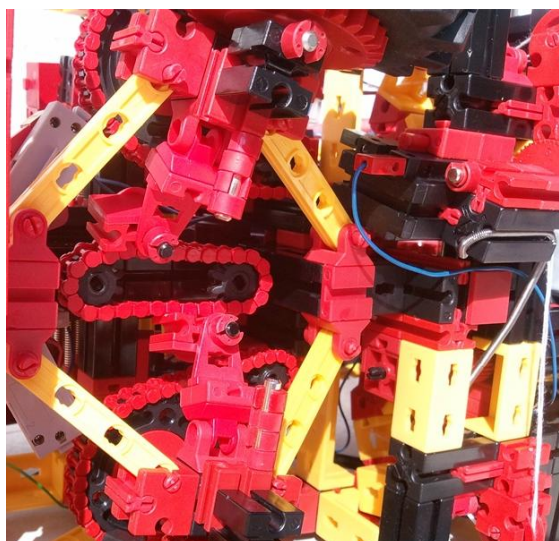
Abb. 7: Lenkung Teleskop-Mobilkran (Stefan Falk)
